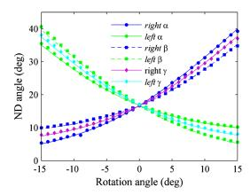
FIG. 3. (Color online) Experimental (points) and calculated (lines) dependences of NLD angles on the NPC rotation angle in geometry from Fig. 1(a). The middle sets of data correspond to NLD from virtual beam.
