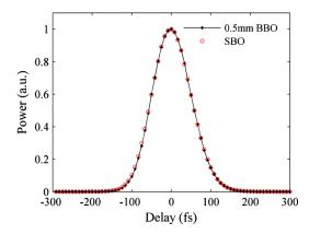
FIG. 4. (Color online) Autocorrelation functions obtained using NPC SBO ( $\tau$ =82.1 fs,  $P_{\rm NLDVB}$ =4.72  $\mu$ W) and 0.5 mm thick BBO ( $\tau$ =81.8 fs,  $P_{\rm BBO}$ =850  $\mu$ W).
