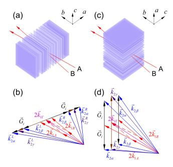
FIG. 1. (Color online) Experimental geometries and corresponding noncollinear phase matching diagrams in NPC of SBO. Input beams lie in the [(a)] and (b)] ab crystallographic plane and in the [(c)] and (d)] bc plane.
