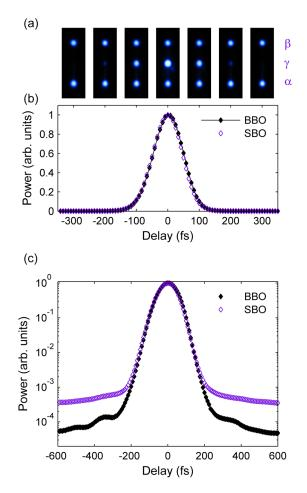
FIG. 3. (Color online) (a) Pattern of the beams with changing delay. (b) and (c) Autocorrelation functions measured using NPC SBO ( $\tau = 77.9$  fs) and 0.5 mm thick BBO ( $\tau = 79.6$  fs) in a linear (b) and logarithmic (c) scales. Attached movie demonstrates nonlinear interaction pattern upon delay (enhanced online) [URL: http://dx.doi.org/10.1063/1.3664094.1].
