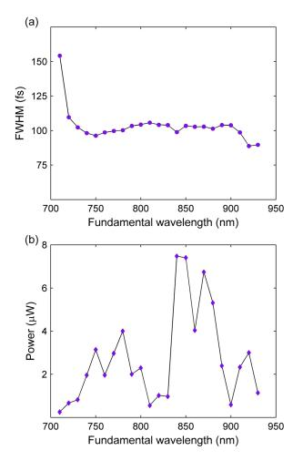
FIG. 4. (Color online) (a) Pulse duration measurement in the tuning range of Ti:Sapphire oscillator at fixed angular position of NPC. (b) Power of auto-correlation signal in the course of pulse duration measurement.
