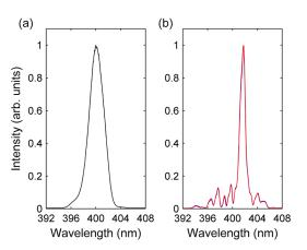
FIG. 2. (Color online) Second harmonic spectra of autocorrelation signal (a) and of single beams (b) obtained using NPC SBO. Both single-beam SH spectra coincide each other.
